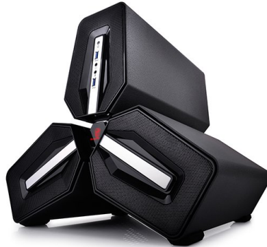
Figure 8: Deepcool Tristellar's unique shape is made possible by using a riser.
