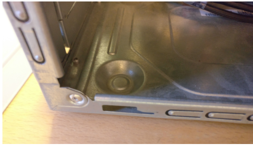
Figure 12: The corner is fastened using a rivet going through two overlapping flanges.
