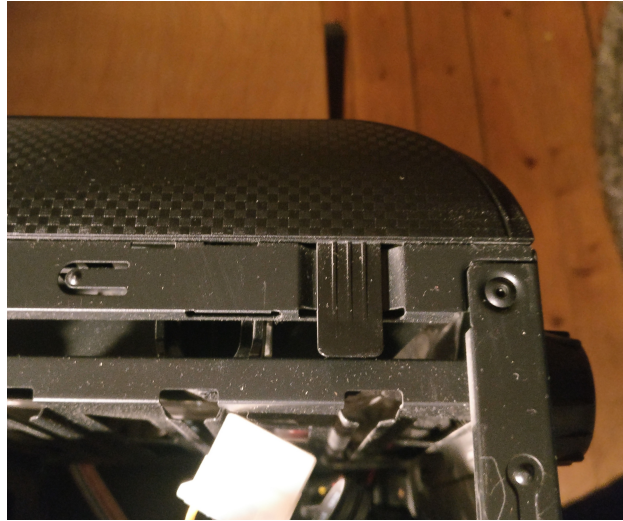
Figure 18: The front piece can be snapped on to the frame.
