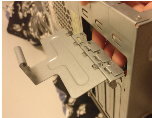
Figure 16: This screwless solution attaches around the edge of the frame, and keeps the cards in place by adding little pins instead of screws.
