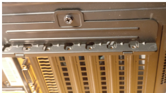
Figure 15: One screw is enough to fasten multiple expansion cards. Behind the fastener, there is some space for the cards to be pulled from the motherboard.
