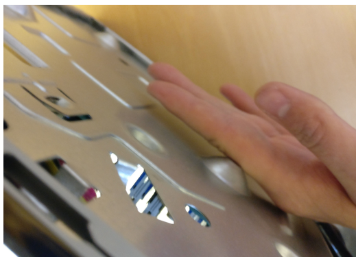
Figure 14: This case used dimples instead of removable standoffs to create a clearance to the motherboard.
