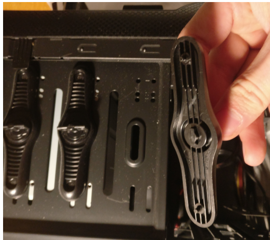
Figure 17: Small plastic pins keep the DVD-drive in place, while the center locks the plastic part to the sheet metal. The drive is only held in place from one side.
